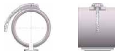
Flachkappe tangential, nur bei DGM/DAK/DMK tangential flat cap, only with DGM/DAK/DMK
